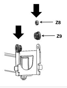
Connect the TV with the TV Plate to the Bracket.
